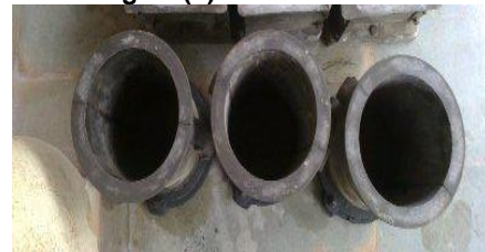
Fig. 3. (c) Cylinder moulds
